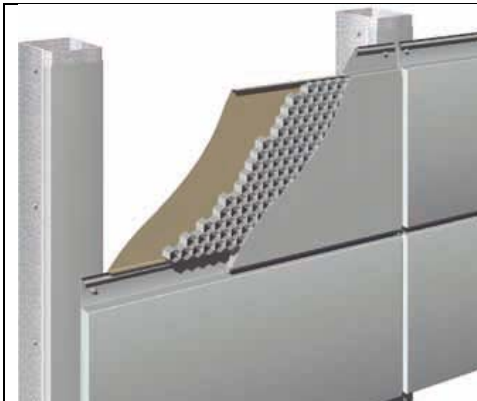
Figure 10: Stratascreen panel with honeycomb core
