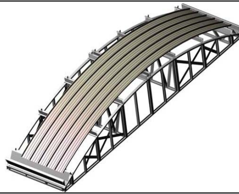
Figure 26: Hi-point as barrel pitched roof
