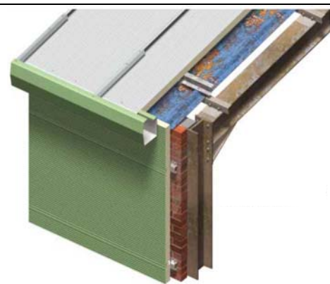
Figure 6: Over roofing of tired steel sheet and over cladding of brick using Kingspan Composite PUR panel
