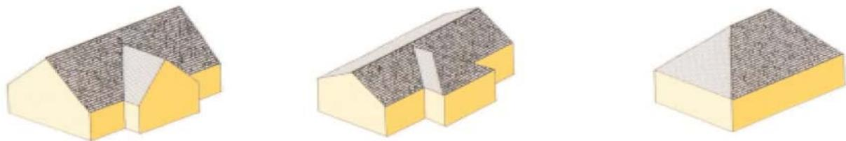
'T' Intersection roof with gable side    Overlaid hip roof with gable side    Hipped roof
