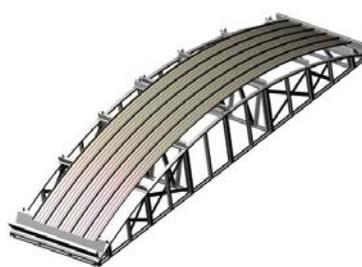
Prefabricated lightweight steel system
