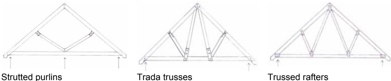
Figure 3: Traditional timber roof trusses
