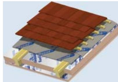
b) Between and under rafter insulation with modern breathable membrane
