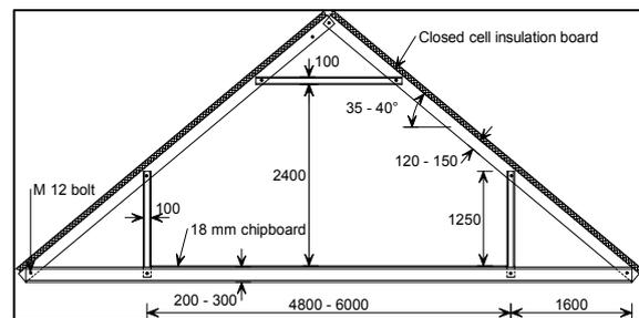
Typical chord and rafter sizes for the open roof system
