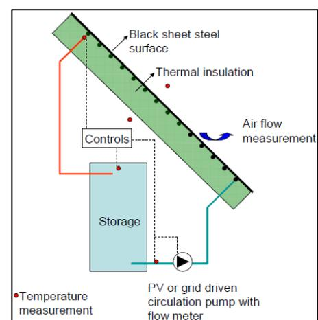
Principle of roof integrated solar
