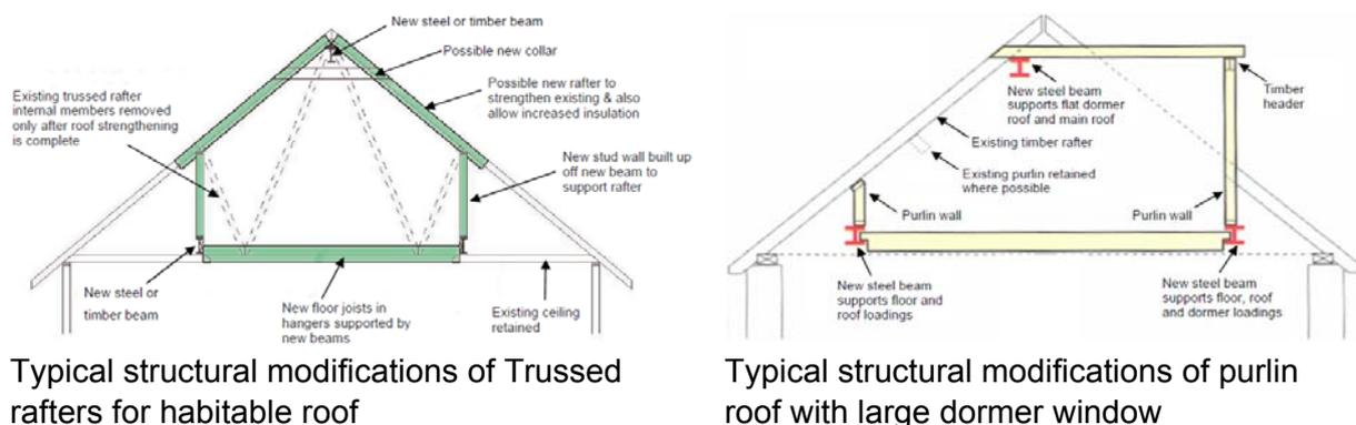
Typical structural modifications of Trussed rafters for habitable roof
