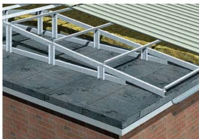
Flat to pitch conversion using lightweight steel
