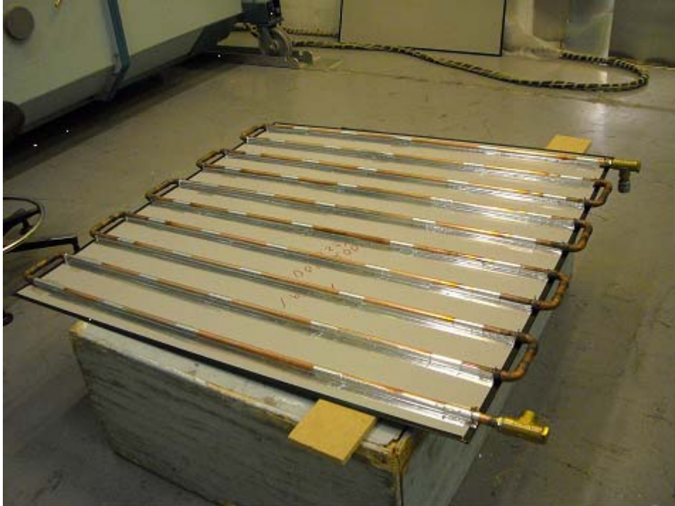
Figure 10. The liquid circulation tubes (copper pipes) attached to external metal sheet with aluminium tape.
