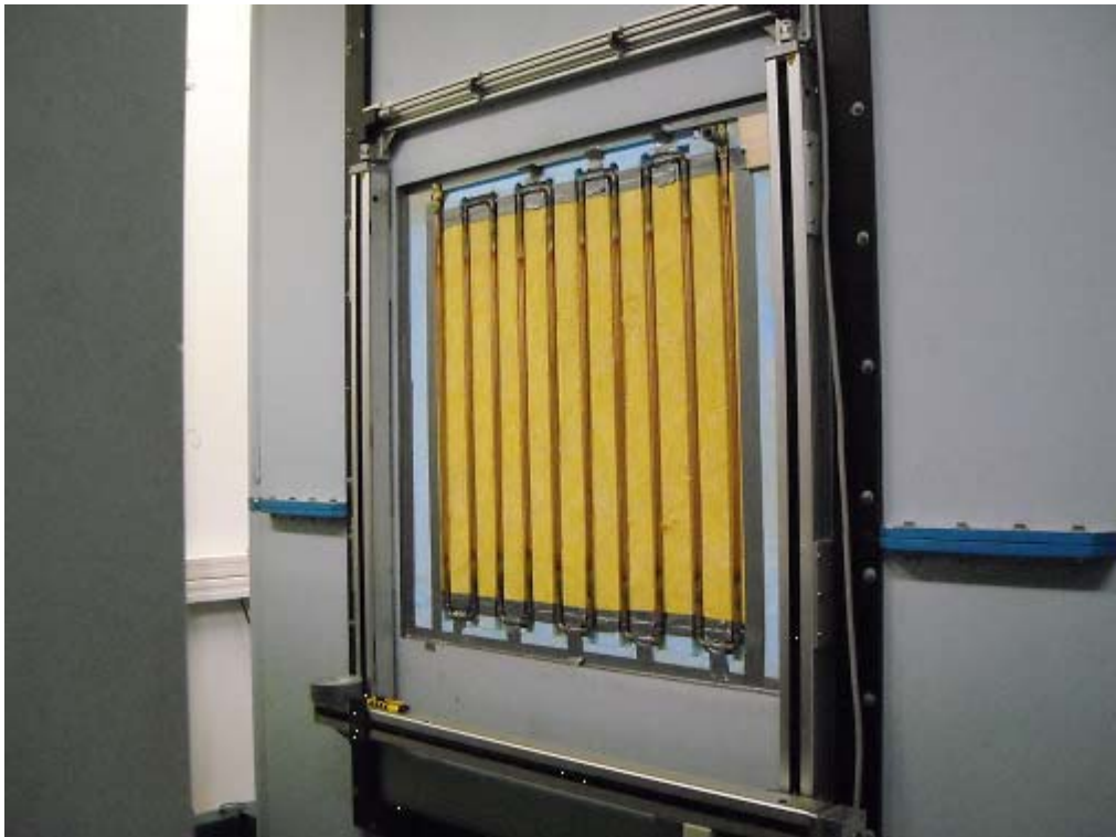
Figure 9. The liquid circulation tubes in the external surface of the thermal insulation.
