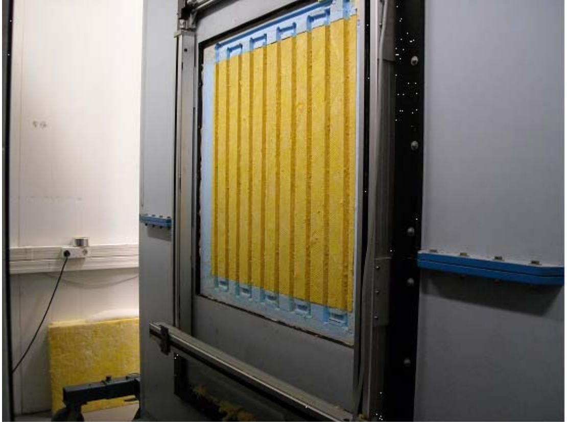
Figure 8. The channels for liquid circulation tubes in the external surface of the thermal insulation.
