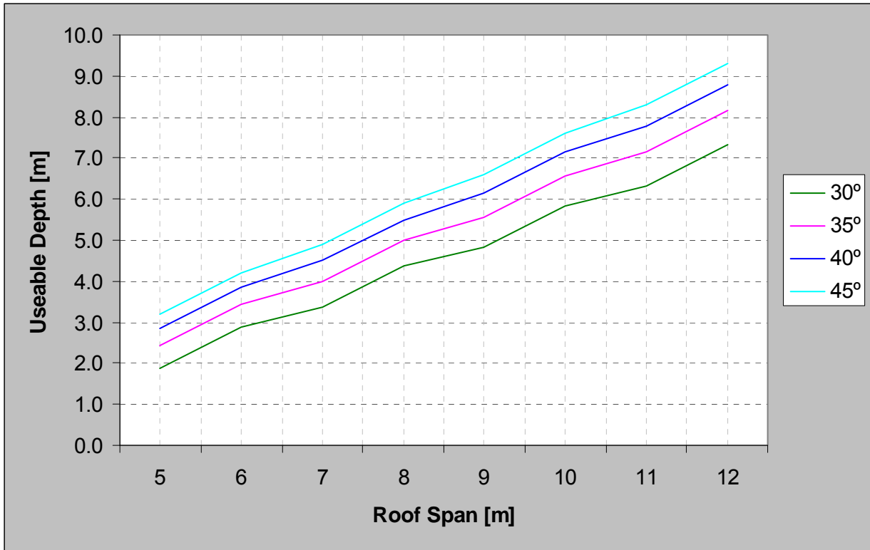
Figure 5: Roof Span Vs Useable Depth
