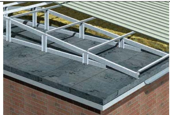
Figure 2: Flat to pitch conversion using lightweight cold form steel and steel cladding
