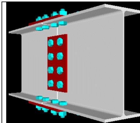
Figure 15: Flange and web plate splice
