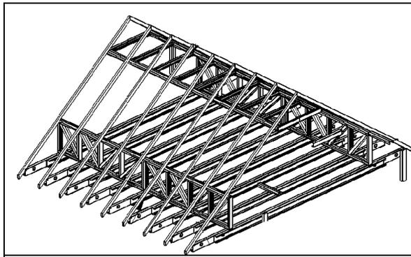
Figure 12: 3D View of lightweight steel solution
