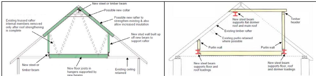
Figure 8: Typical structural modifications of Trussed rafters for habitable roof
