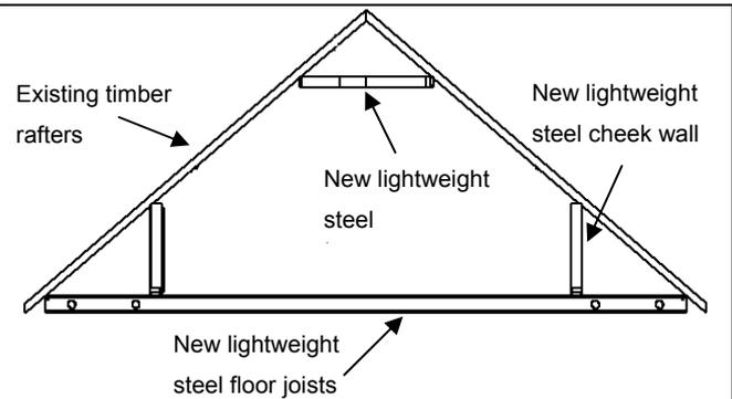
Figure 13: Cross section view of lightweight solution
