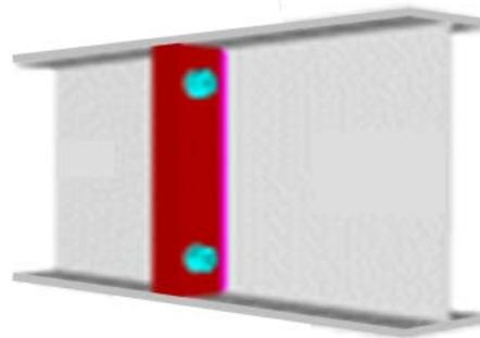
Figure 16: End plate splice
