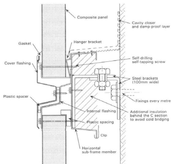
*Figure 11: Joint detail in prototype steel over-cladding system*
