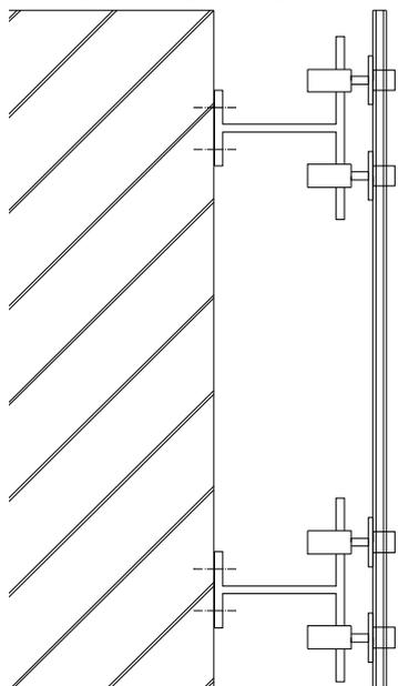
This is not a real steel-intensive solution, but it's quite interesting. The principle is to create a new glass façade, with a dynamic air space between the wall and the glass. This air space is opened during summer, and there is a natural air flux. In winter, this space is totally closed, so an extra insulation layer is obtained.
